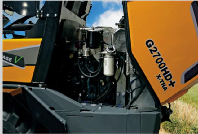
Performing maintenance to the G2700 is no problem at all because the service points are easy to reach. Filters, hydraulic system and engine can be freely accessed via the easy-to-open bonnet, tilting cab or other service panels. This ensures that daily checks and maintenance can be carried out quickly and in a safe manner.
