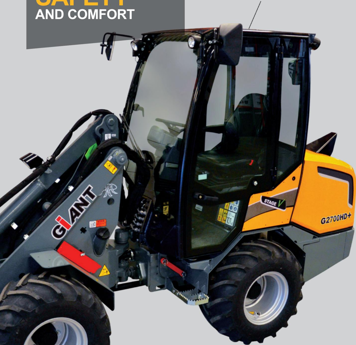
In the cabin, a comfortable working environment has been created so long working days are no problem. The steering column is fully adjustable and all necessary information can easily be read from a central display. While using the joystick, the operator can rest his arm on an ergonomically shaped armrest. All key functions are close to the joystick so that they can be operated without effort. Optionally, the machines can be supplied with items that are desirable for the work to be performed.
