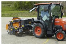
Two disc brushes mounted in front of the axle transport the debris to the centre of the MSH. The roller brush, located behind the axle, brushes the debris into the large-volume hopper.
