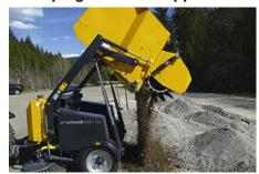
The MSH trailer sweeper series has a steel hopper with a 1.5m<sup>3</sup> capacity and a discharge height of 1,800mm. The hopper is tipped hydraulically at the back.
