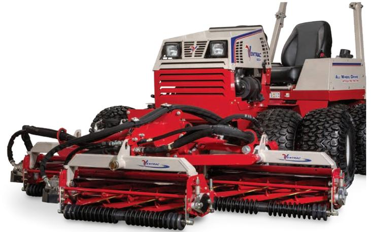
Ventrac's Triplex Reel Mower features a 74-inch cutting width and is designed to be the ultimate trim and surround mower.
