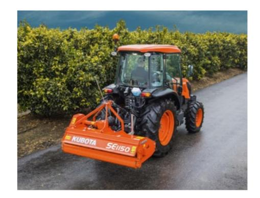
More power and performance for all tasks is the motto for the lift linkage of the M5001N. Thanks to its stable category II 3 point hitch, the tractor can lift heavy equipment with ease. 2,300 kg lifting capacity speak for themselves. You will really appreciate the additional lifting capacity in areas where your previous tractor reached its limits.
