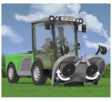
Efficient lawn moving The knives rotate in opposite direction
