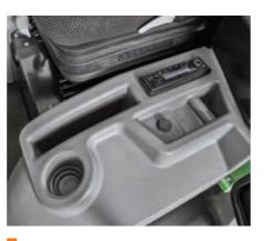
Storage facilities On the left side a cup holder, power outlet and storage facilities adds to a good working environment. The optional radio is also placed here.
