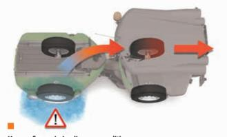
**Keep a firm grip in slippery conditions** If you loose grip on one wheel the 4WD ensures that power is automatically transferred to the opposite wheel crosswise meaning, that if you loose grip on the rear right wheel the power will be transferred to the left front wheel and vice versa.
