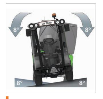
Strong articulation point The strong articulation point allows for an oscillating movement between front and rear chassis of +/- 8 degrees.
