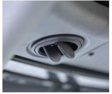
Air ducts The strategically placed air ducts are easily adjusted to suit the air circulation needs in the cabin.
