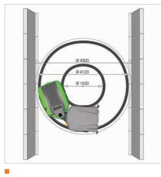
**High manoeuvrability** The City Ranger 3070 is articulated making it highly manoeuvrable in tight spaces. The inside turning circle of the basic machine is only 1650 mm.
