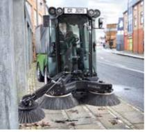
Sweeping narrow passages with a 3rd brush The 3rd side brush is equipped with a springloaded and collision-proof function, increasing the service life of the brush while also safeguarding surrounding objects. The tipping function is controlled via the cabin joystick and the hydraulic system of the machine and can advantageously be activated when encountering depressions, gutters, kerbstones, and the like.
