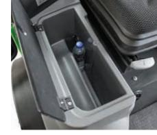
Air cooled glove box On the right side of the seat there is a closed glove compartment. This has an air duct in it, which helps keep a lunch box or a drink cooled during the day.
