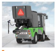
High pressure washer and wander hose For extra cleaning functions, the hopper can be equipped with a high pressure washer with hand lance and a 5 metre wander hose.
